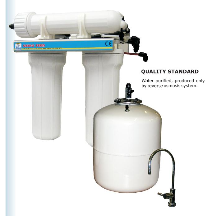
OSMO FEED is a water purifying and de-mineralising system destined specifically for technical use. It is able to produce de-mineralised water using the reverse osmosis method, obtaining a desalination level greater than 90% and a specific conductivity at 25°C not greater than 30 microS/cm.
